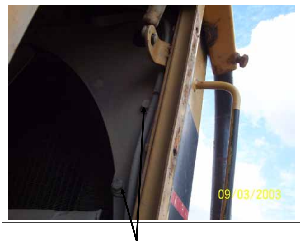
Condenser frame mount bolts left side
