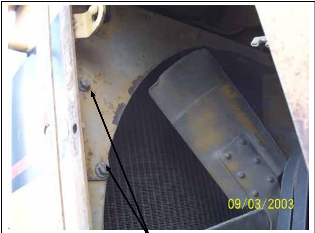
These bolts are removed and then reinstalled to hold the condenser frame
