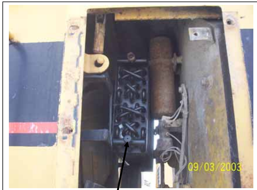
Condenser frame in place. Install separate of condenser coil for easy fit.
