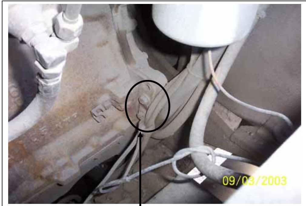
Drier and bracket installed. The existing lines may have to be moved aside a bit.
