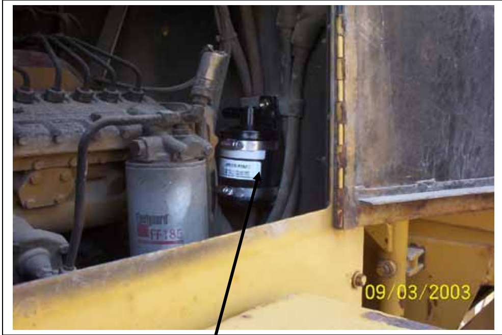
Drier and bracket installed. The existing lines may have to be moved aside a bit.
