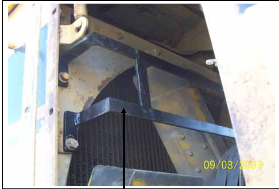
Condenser frame in place. Install separate of condenser coil for easy fit.
